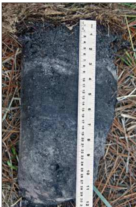
Figure 21. Example of indicator S9 (Thin Dark Surface). Scale in inches on right.
