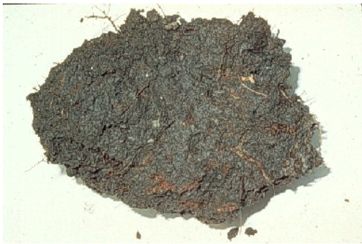
Figure 5. Soil showing matrix (brown) and mottles (reddish-brown)
