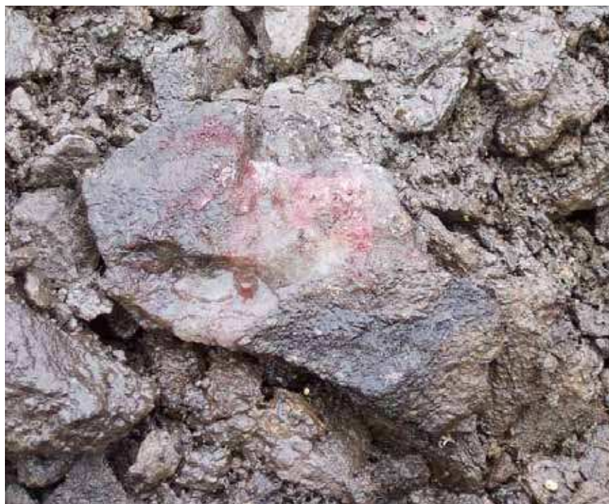
Figure 54. When alpha, alpha-dipyridyl is applied to a soil containing reduced iron, a positive reaction is indicated by a pink or red coloration to the treated area.
