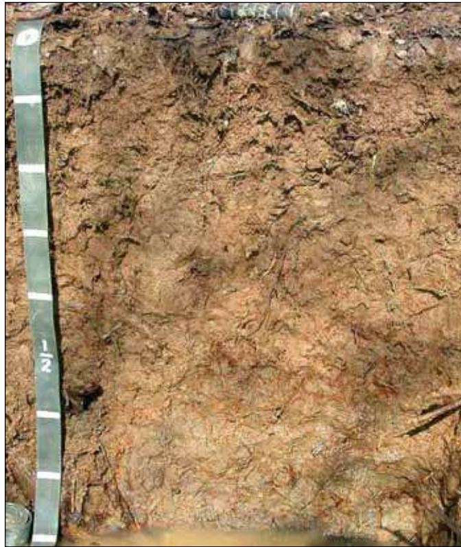
Figure 29. The Piedmont Floodplain Soils indicator is restricted to floodplains that are actively receiving sediments and groundwater discharge with high iron content. Photo by M. Rabenhorst. Scale in 4-in. (10-cm) increments.
